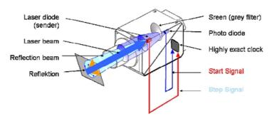
Laser-Distance measuring by "Time of flight" technology
