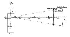
The software either converts polar coordinates of a measurement point to orthogonal X and Y coordinates or presents a profile (table of X, Y-values) for each sweep from one side to the other. Within the application program the user can specify the seize of the Y increment and thus the length of the output table containing the profile data.
